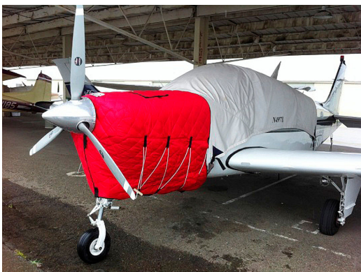
Beech Bonanza Insulated Engine Cover, fully enclosed
