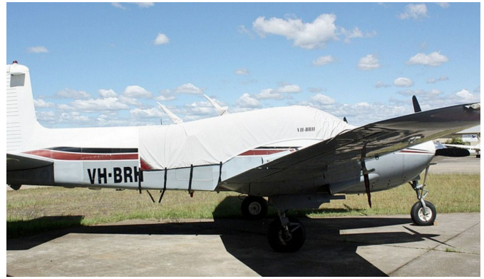
Twin Bonanza Canopy Cover, extends to cover air stair.
