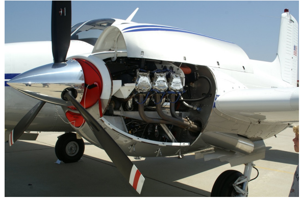
Beech Twin Bonanza Engine Inlet Plugs
