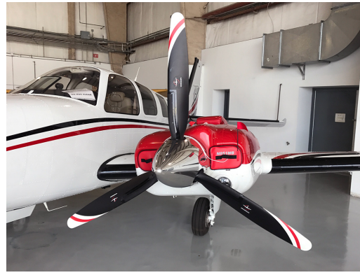
Beech Baron 58 Engine Inlet and Cowl Top Plugs, With A/C (G58 Models)
