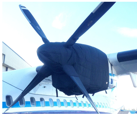
ATR-72-202 Insulated Engine & Prop Hub Covers
