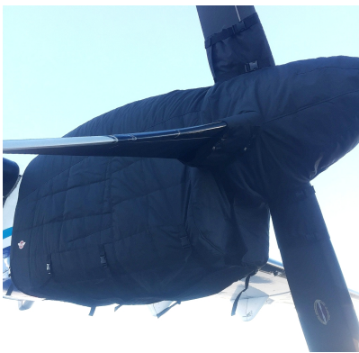
ATR-72-202 Insulated Engine & Prop Hub Covers
