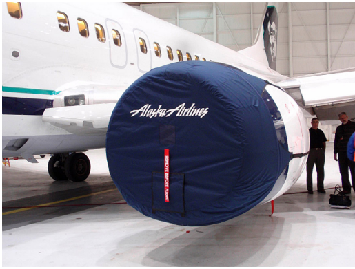
Boeing 737 Intake Covers with w/ Pre-heating hose access vent & attachment detail
