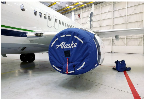
Boeing 737 Intake Cover w/ Heater Attachment
