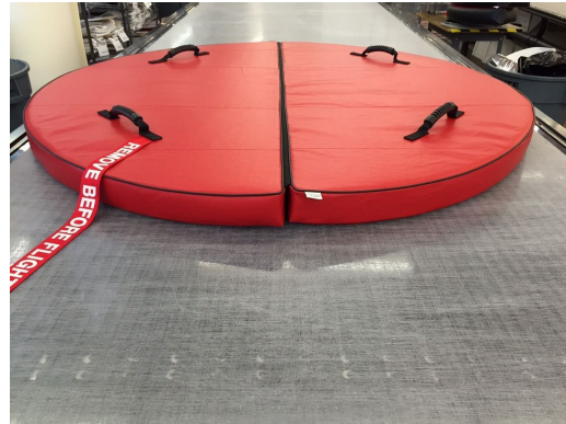
Boeing 737 Max Intake Plug, folding type
