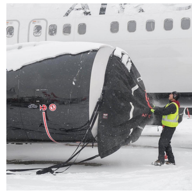
Intake Cover w/ heater hose attachments for cold weather.
