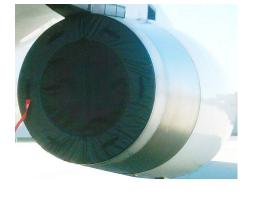
Airbus A330 Intake Plug, framed bi-fold type
