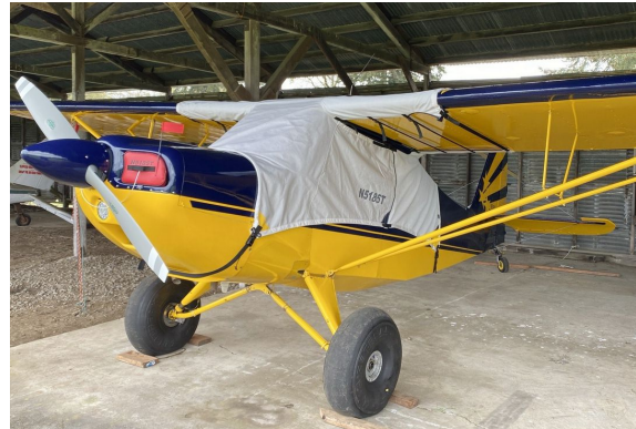
American Champion Citabria canopy cover over the top style, extends to cover gas caps, Engine Plugs
