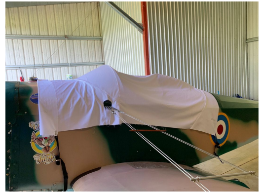
Bowers Flybaby Canopy Cover, test fit design
