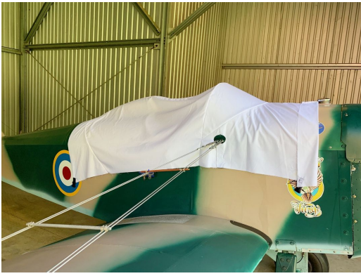
Bowers Flybaby Canopy Cover, test fit design
