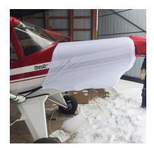
Bearhawk Engine Cover (test fit), Insulated Prop Cover
