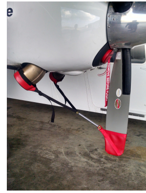
Britten-Norman Islander, prop tie/exh. cover and inlet plug for BN-2T Allison Engines.
