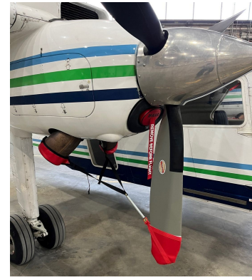
Britten-Norman Islander Engine Inlet Plugs & Prop Tie
