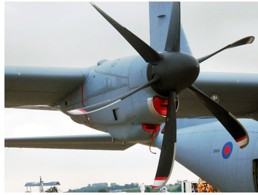
Main and Oil Cooler inlet plugs
