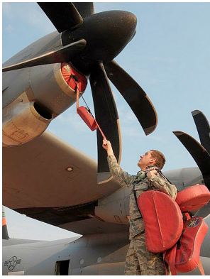
C-130 Engine and Oil Cooler inlet plugs
