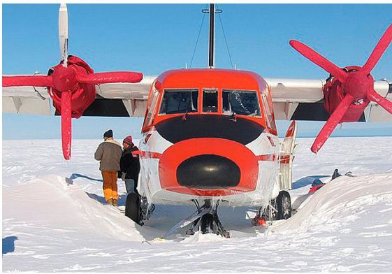
Casa 212 Insulated Engine & Propellor/Spinner Covers
