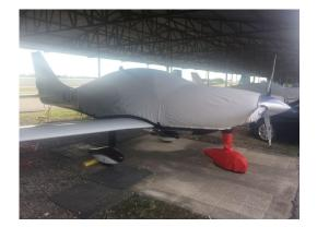
Lancair Columbia Extended Canopy/Engine Cover, Nose Wheelpant Cover
