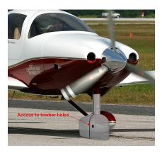
Nose Wheelpant/Strut Cover (illustration)
