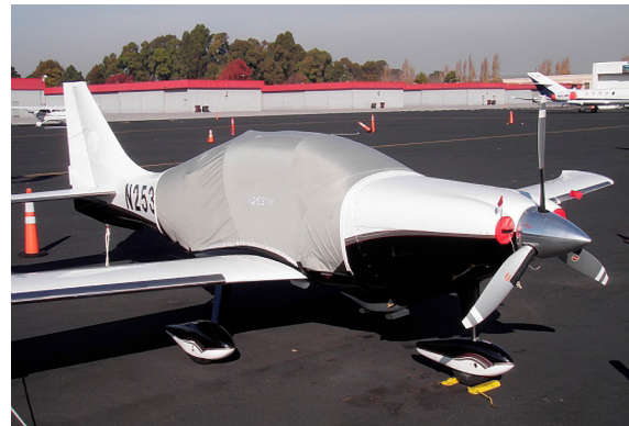
Cessna Corvalis Extended Canopy Cover & Engine Inlet Plugs
