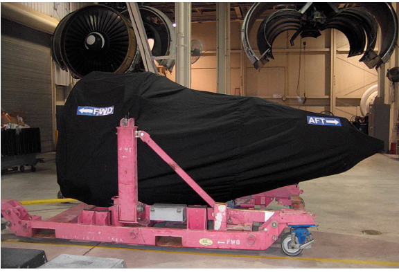
CFM-56-7 Off-link Engine Shipper/Transport cover, w/ Exhaust Cone, fully enclosed
