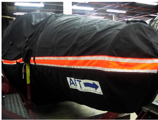
CFM-56-5A/5B Off-link Engine Shipper/Transport cover, w/ Exhaust Cone, fully enclosed
