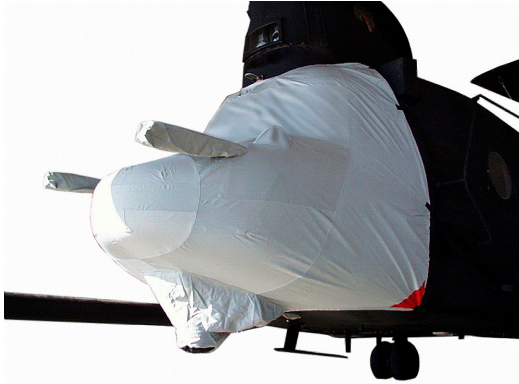
Spec. Op's CH-47: refuel boom, FLIR dome
