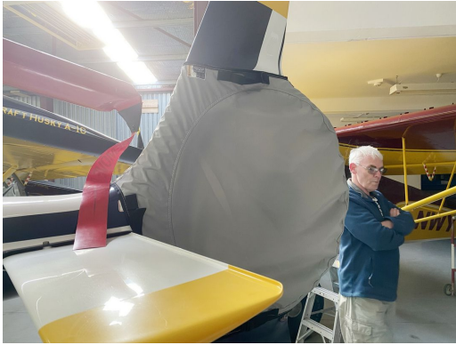
Guimbal Cabri G2 Tailfan Housing Fenestron Cover
