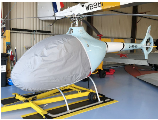
Cabri G2 Light Weight Travel Bubble Cover Robinson R-22 Insulated Engine Cover (also covers bottom) & Front Blade Tie-down
