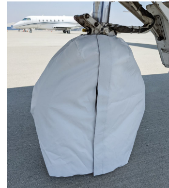
CJ1 Nose Gear Tire Cover, test fit
