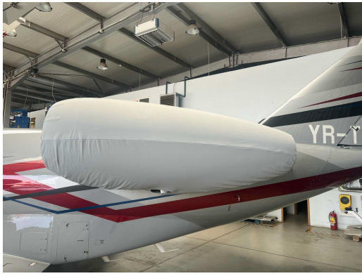
Citationjet 525C, CJ4, Complete Nacelle Cover, light weight Spandex
