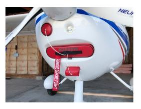
Flight Design CTSW, CTLS, 2K & MC Engine Inlet Plugs
