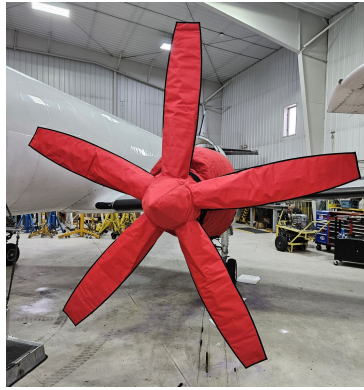
Fairchild Metro 5 Blade Insulated Insulated Prop Covers
