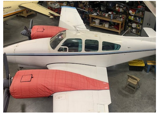
Beech Baron B55 Insulated Engine Covers
