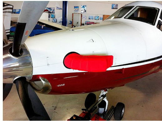
Pilatus PC-12 Prop Cover, Prop Tie/Exhaust Cover Pilatus PC-12 Exhaust Cover, Fully Enclosed, for protection against corrosion.
