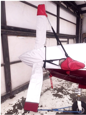
Pilatus PC-12 Prop Cover, Prop Tie/Exhaust Cover Pilatus PC-12 Exhaust Cover, Fully Enclosed, for protection against corrosion.
