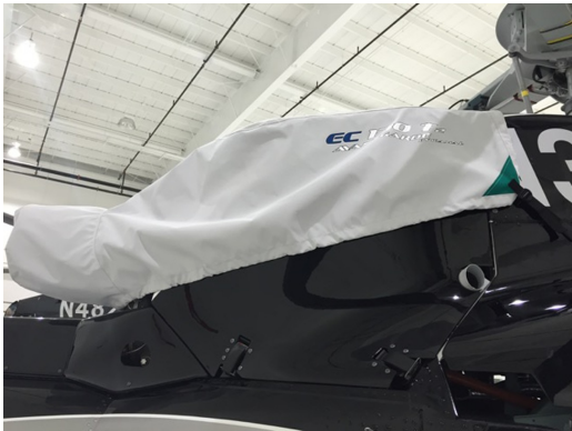
EC-130 Engine Area/Exhaust Cover
