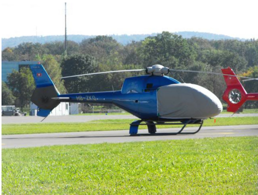
EC-130 Bubble, Tailfan, and Rotor Hub Cover
