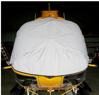
EC-135 Windshield/Skylights Cover, pinches in door jambs Bubble Cover w/ nose mounted radome, Upper Deck Plugs/Cover
