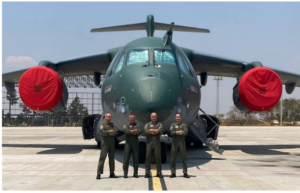
Embraer C-390 Millennium Intake/Exhaust Covers
