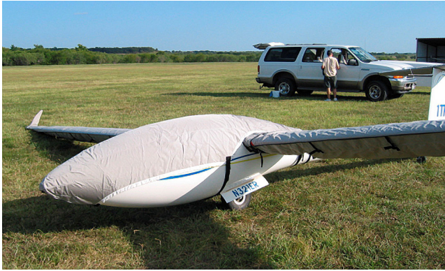
Canopy/Nose Cover, Wings and Horizontal Stab Covers
