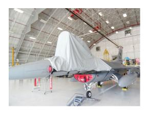
McDonnell Douglas F16-D Canopy Cover, open cockpit type (test F-16 CANOPY COVER, OPEN POSITION (C-Model, single fit cover)
