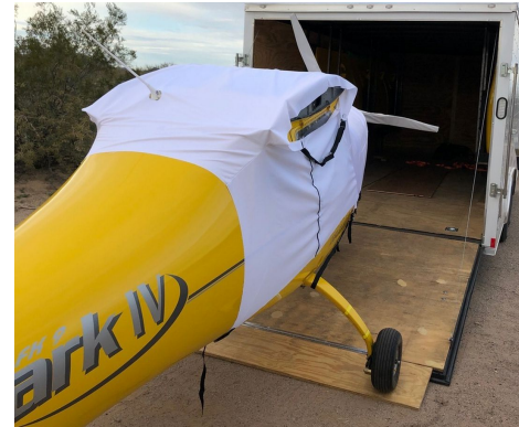
FK-Lightplanes FK-9 Canopy Cover, test fit cover
