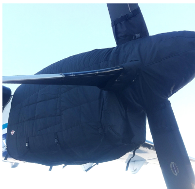
ATR-72-202 Insulated Engine & Prop Hub Covers
