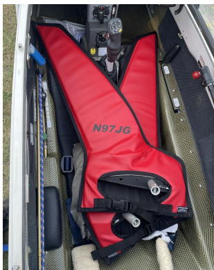
Schempp-Hirth Ventus-2B winglet/wingtip pads
