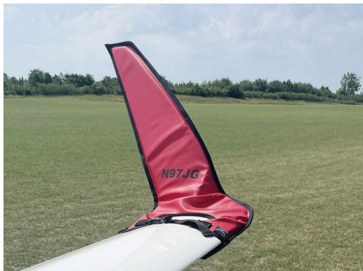
Schempp-Hirth Ventus-2B winglet/wingtip pads
