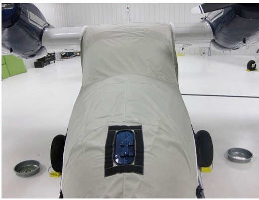
Grumman Widgeon Cockpit/Nose Cover, tie-down cleat detail
