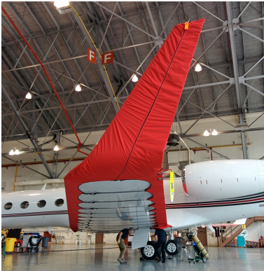
Gulfstream G550 Wing/Winglet Covers
