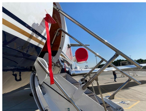
Grumman Gulfstream G-IV SP Pitot Cover
