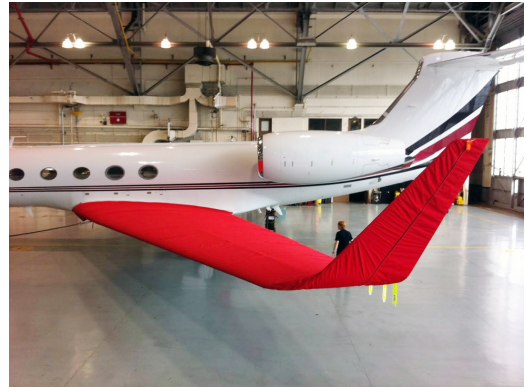
Gulfstream G550 Wing/Winglet Covers
