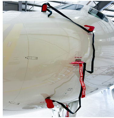
Gulfstream G500 FOD protection plugs for mfg process Gulfstream GVII Pitot Probes/TAT/Ice Detector Set, Heat Resistant Type
