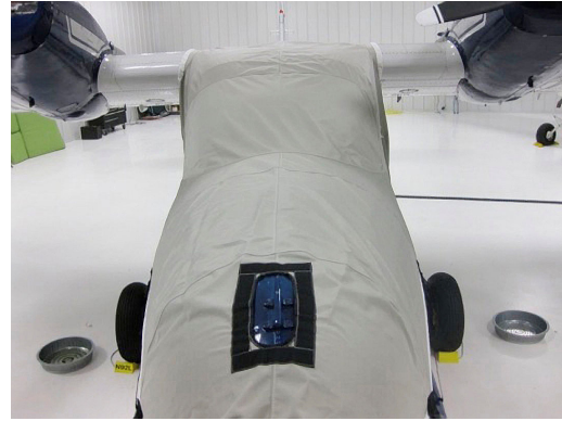
Grumman Widgeon Cockpit/Nose Cover, tie-down cleat detail
