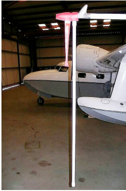
Grumman Mallard Pitot Cover with Install Tool
