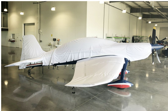
Gamebird GB-1 Extended Canopy/Engine, Wing & Empennage Covers (test fit covers) Gamebird GB-1 Extended Canopy/Engine Cover, 3D model
