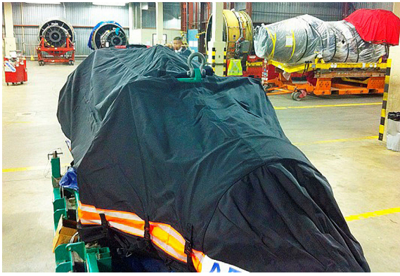
GE CF-3GE CF-34 QEC Engine Long-term Storage/Transport Cover "Bag"4 QEC Engine Long-term Storage/Transport Cover "Bag"
