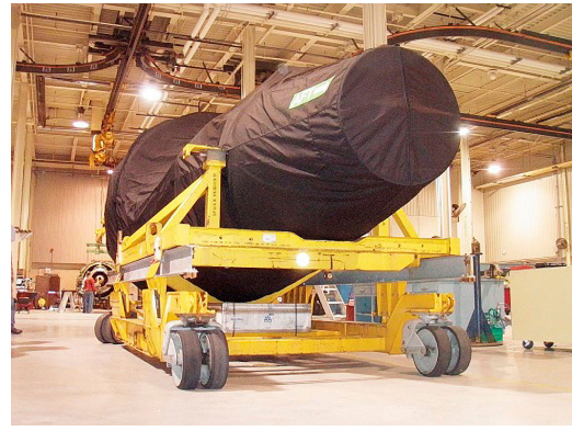
GE CF-6 QEC Engine Long-term Storage/Transport Cover "Bag" (Boeing 767)
