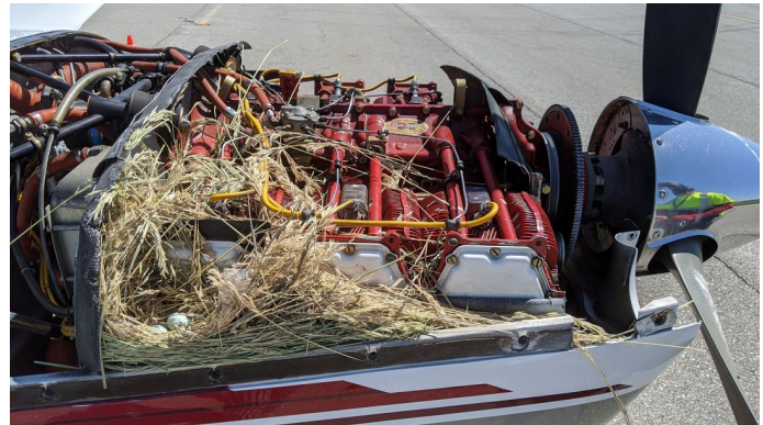
ENGINE PLUGS PREVENT BIRD NEST FOD. Piper Saratoga Engine Cowling Bird's Nest
