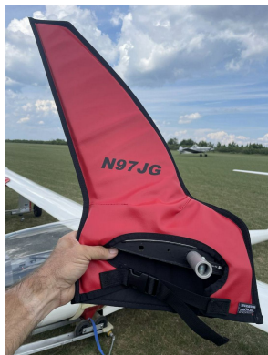
Schempp-Hirth Ventus-2B winglet/wingtip pads
