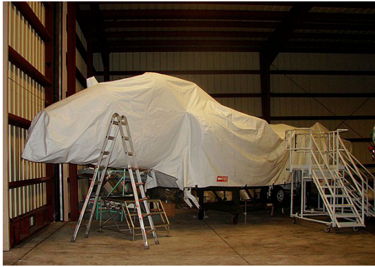
GR-7/9 FULL FUSELAGE COVER , NSN's: 1730-01-600-4557 & 1730-01-600-6757, dual seat
