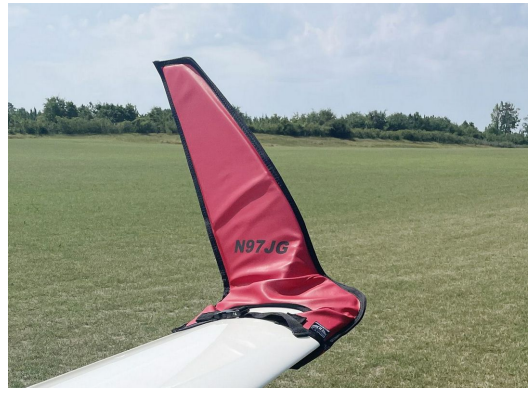
Schempp-Hirth Ventus-2B winglet/wingtip pads
