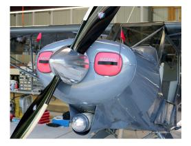
Piper PA-18 Super Cub Engine Inlet Plugs
