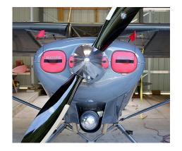
Piper PA-18 Super Cub Engine Inlet Plugs
