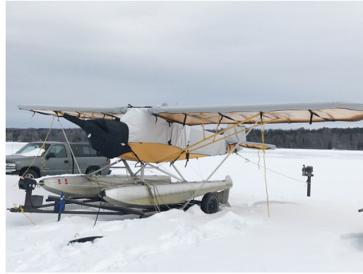
Piper J-3C-65 Cub Engine Cover, Fully Enclosed Piper J3 Cub Extended Canopy, Wings, Empennage & Insulated Engine Covers
