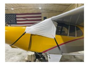
Piper J5A Windshield/Skylight Cover, test fit
