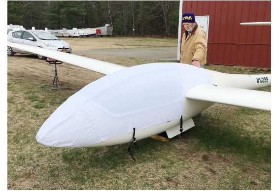
Grob 102 Astir CS Canopy/Nose Cover (test fit)
