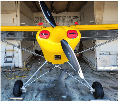
Preceptor STOL King Engine Plugs ENGINE PLUGS PREVENT BIRD NEST FOD. Piper Saratoga Engine Cowling Bird's Nest
