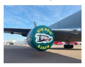
Boeing KC-135 Intake Covers, soft type, CFM56 engines
