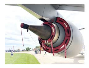
Boeing KC-135 Bypass and Exhaust Plugs
