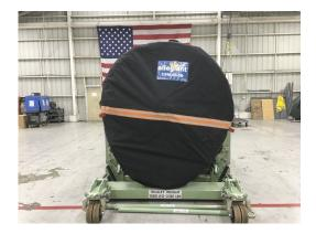
CFM56-5B Off Link Cover, fully enclosed
