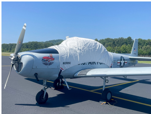
Navion L-17B Canopy Cover (With Avionics Bay Extension)
