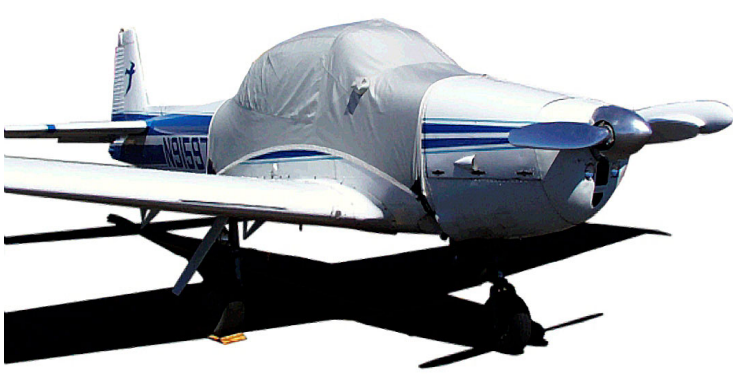
Navion Canopy Cover extends forward to firewall line.
