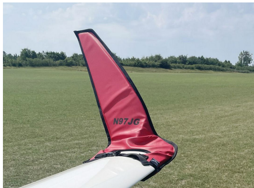
Schempp-Hirth Ventus-2B winglet/wingtip pads
