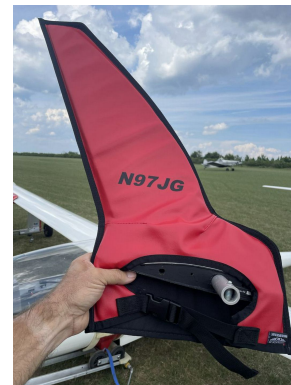
Schempp-Hirth Ventus-2B winglet/wingtip pads
