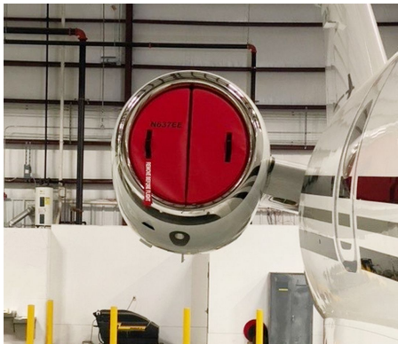
Embraer Legacy 500 Engine Inlet Plugs, folding type
