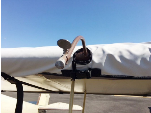
Luscombe 8A-8F Silvaire Wing Covers, Pitot Tube detail.
