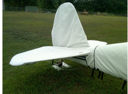
Luscombe Empennage Cover, two-piece design
