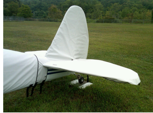
Luscombe Empennage Cover, two-piece design
